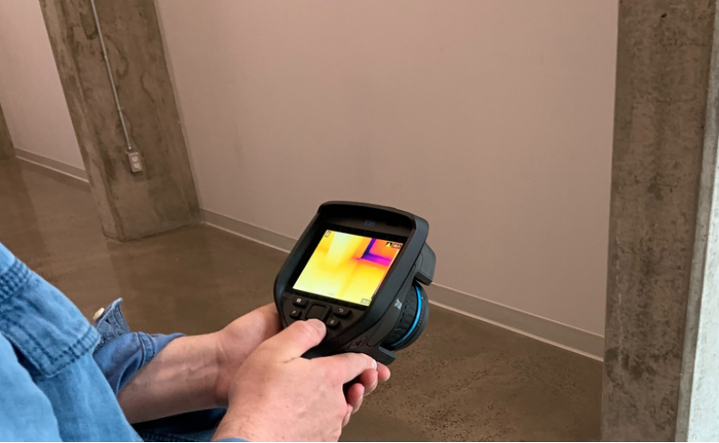
PHOTO 1. THERMAL IMAGING AT DALHOUSIE BUILDINGS
