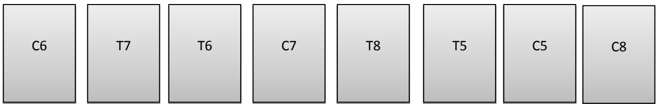
Figure 2.2.2: Schematic of the PV set-up on both locations: Dalhousie University & Dartmouth Residential Neighbourhood. Note the figure is not to scale; it is showing the location of the control and treatment panels where T= treatment and C=control
