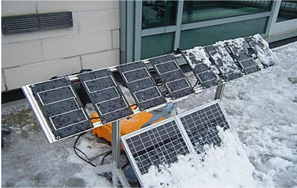
Snow & ice cover on the PV setup on the Rowe Building. Note the variability in percent cover and snow characteristics
