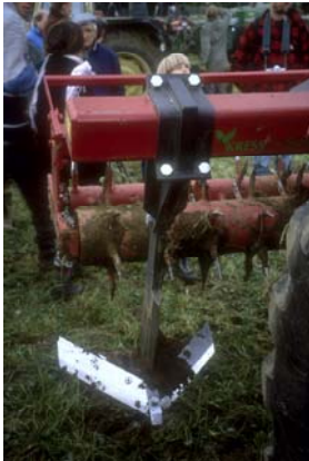
Figure 12 – The Walter Kress quackgrass harrow, which combines stubble ploughing with culling (photo: Denis La France).
