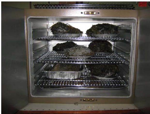
Figure 8. Drying oven used to calculate dry biomass of algal samples.
